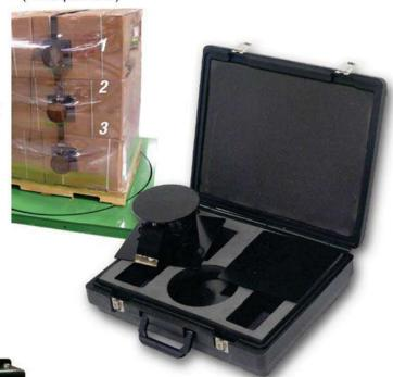
Quickly change from containment force testing to puncture resistance tests
